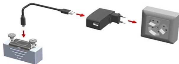
*The battery is charged via the sensor's USB-C port.*
