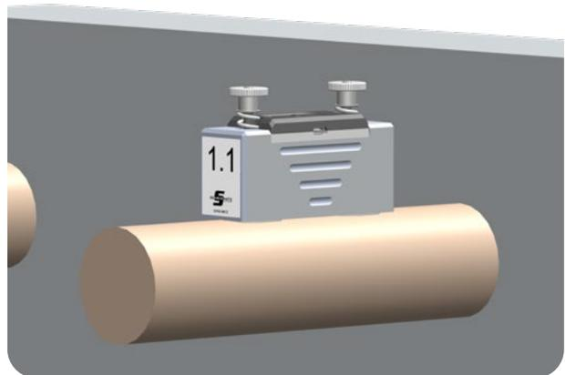
5. Placement validation - If the magnets do not automatically jump onto the measuring surface, press down the knurled nuts one after the other. The magnets should now jump onto the surface. The attraction force of the magnets is now optimal.
