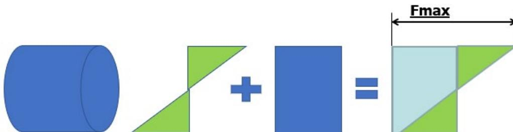
With 4 QE2008-W sensors mounted around the circular beam, it is immediate to measure the total maximum tension on the beam. In addition, this mounting configuration allows to extrapolate the direction in which the bending occurs.
