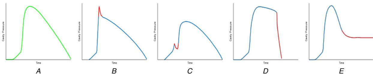
A peak in the pressure profile, like the one shown in Figure B, denotes a late switch to the holding phase and/or a high injection speed. Figure C implies an early switch to the holding phase. A short duration of the holding phase reflects on the cavity pressure profile like shown in Figure D. Lastly, in Figure E a residual pressure is shown.
