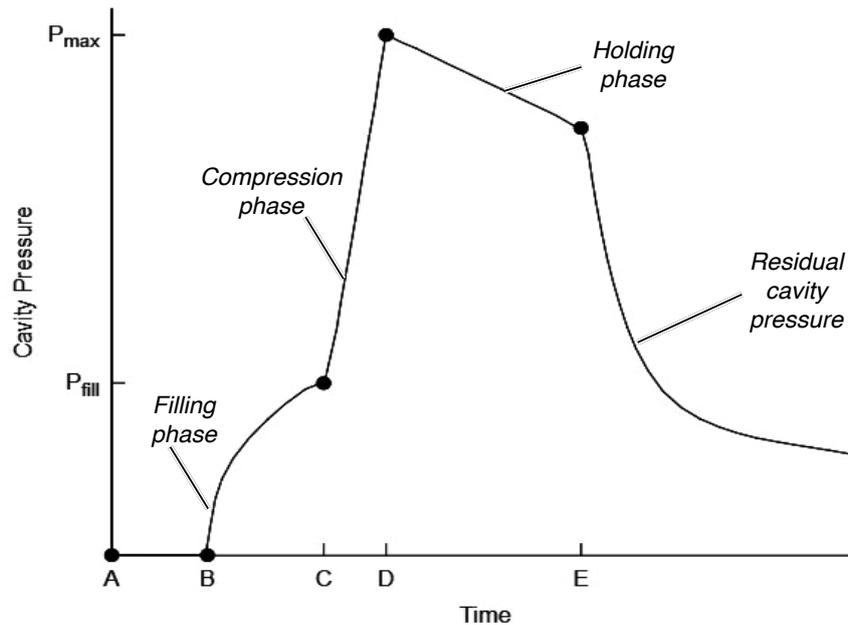
A correctly shaped pressure transition between phases implies a high quality part produced. Moreover, a correct setup will allow the machine run with lower energy consumption and faster cycle times. On the other side, a bad setup can cause serious damages on the involved machine parts.
