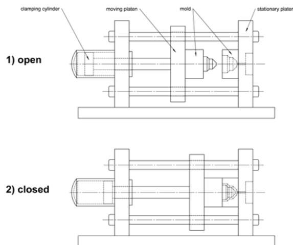
When the press is closed (the moving platen is compressing the object), the applied force causes the two stationary platens to slightly translate away from each other, making the tie bars elongate.
