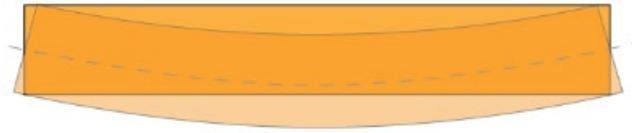
The bottom surface of the beam gets longer in length, while the top surface of the beam gets shorter in length. Also, along the center of the beam – also known as the neutral axis –, the length doesn't change. The bottom surface is under tension, while the top surface is under compression. Furthermore, the displacement of the beam varies linearly from the top to the bottom – passing through zero at the neutral axis.
