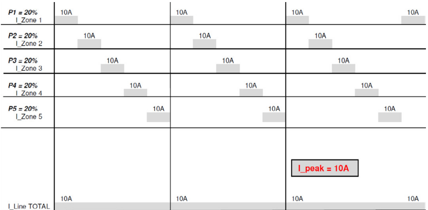
Fig. 2 With Power Distribution, without Power Limit
