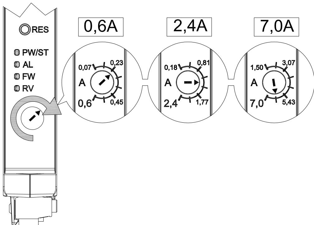
Once the movement of the rotary selector is finished, the PW / ST LED will flash BLUE a number of times equal to the number of the selected position to confirm the selection of the motor size made
