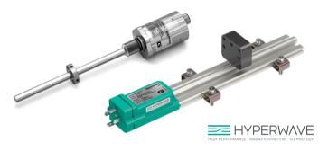
Absolute contactless linear position transducer with HYPERWAVE magnetorestrictive technology, with analog output interface. The absence of electrical contacts on the magnetic slider eliminates wear on the moving parts and guarantees a theoretically infinite lifespan. Total protection with ideal use even in difficult environments with high levels of dust and percolating liquid contamination. Excellent linearity, repeatability and resistance to mechanical vibrations and shocks.
