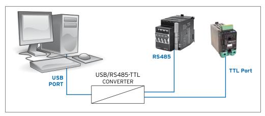
This connection requires a USB/RS485-TTL converter and connection cables for connection between the PC on which GF\_eXpress is installed and the device to be configured.
