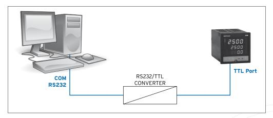
This connection requires a RS232/TTL converter and connection cables for connection between the PC on which GF\_eXpress is installed and the device to be configured.
