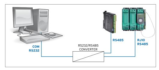
This connection requires a RS232/RS485 converter and connection cables for connection between the PC on which GF\_eXpress is installed and the device to be configured.
