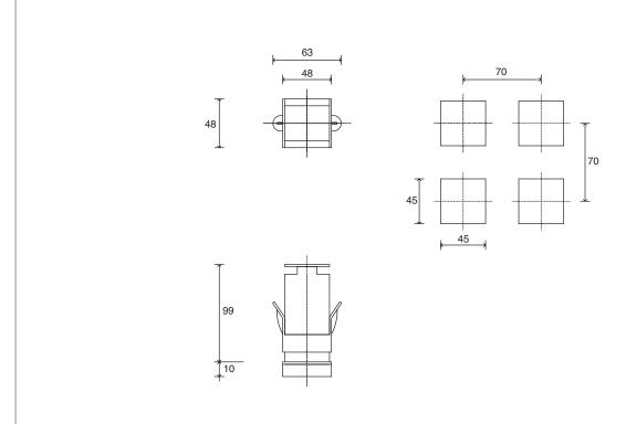
Dimensions: 48x48mm (1/16 DIN) depth 99mm
